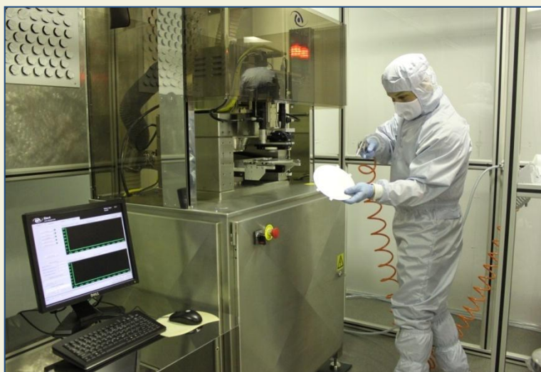
Line width — 10 nm, wafer diameter — 150 mm
